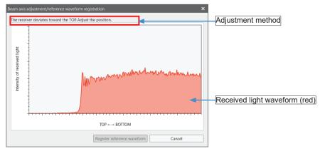
2. If the beam axis is aligned according to the displayed adjustment method, the waveform will be displayed in blue and the message "Reference waveform can be registered" will be displayed.
