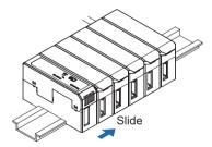
3. Attach end plates MS-DIN-E (optional) with the flat side facing in so as to enclose the connected units at the ends.
