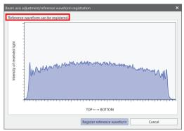
3. If you successively register a reference waveform, click Register reference waveform. The received light waveform displayed in the graph window will be registered as the reference waveform.
