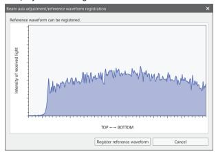
If the beam axis is misaligned, the waveform will be displayed in red. The adjustment method is displayed on the top left of the window. Move the emitter or receiver upward, downward, rightward, or leftward according to the instruction displayed in the dialog box. For details on how to adjust the beam axis, refer to "5.3.2 Adjusting the Beam Axis" in the **HG-T** User's Manual.
