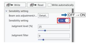
2. For stable measurement of objects with high transmittance, you must increase the judgment level. For the judgment level, you can use either numerical input or slider input.
