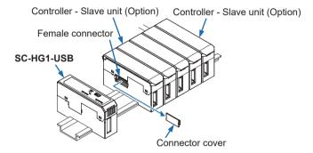
Note: Keep the connector cover removed from the controller in a safe place.
